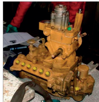
A fuel pump worn out by cavitation
