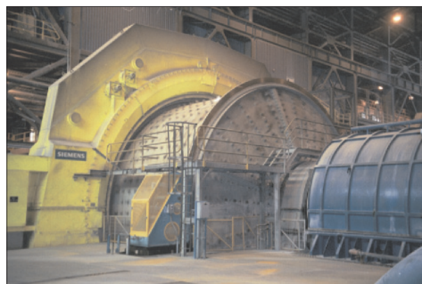
SAG Mill usually employed by mining company in Chile.
